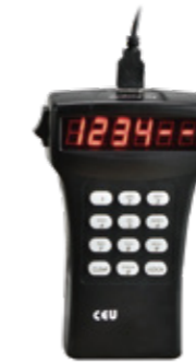
Electronic handheld override for no battery power opening and audit functions
